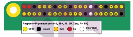
The Raspberry Pi GPIO header is made up of 40 male pins. Some pins are available for you to use in your physical computing projects, some pins provide power, while other pins are reserved for communicating with add-on hardware like the Sense HAT (see **Chapter 7**).
