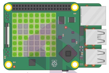
▲ Figure 7-16: Displaying an image on the matrix
