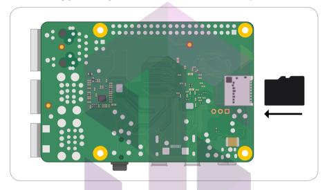
The microSD card will slide into the connector, then stop without a click.
