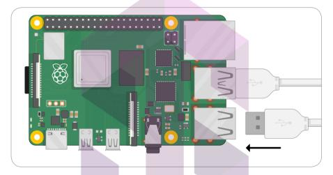
The USB connectors for the keyboard and mouse should slide home without too much pressure; if you're having to force the connector in, there's something wrong. Check that the USB connector is the right way up!
